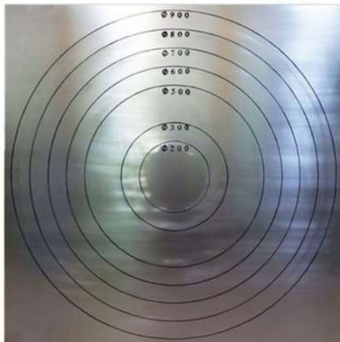
Figure 2.1 – Slump spread test base plate
